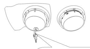
Turn the knob until the locking mark aligns with the Open/Close Index. Insert the knob lock key into the lock hole, and turn it clockwise by 180 degrees to activate the knob lock.
